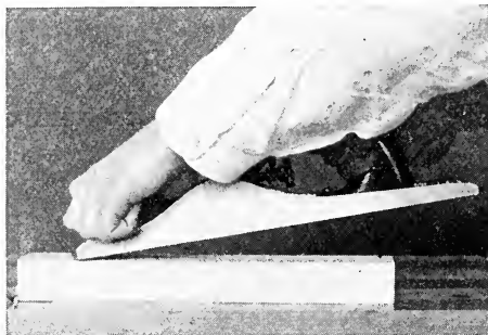
Fig. 38—Lifting Plane on Return Stroke
